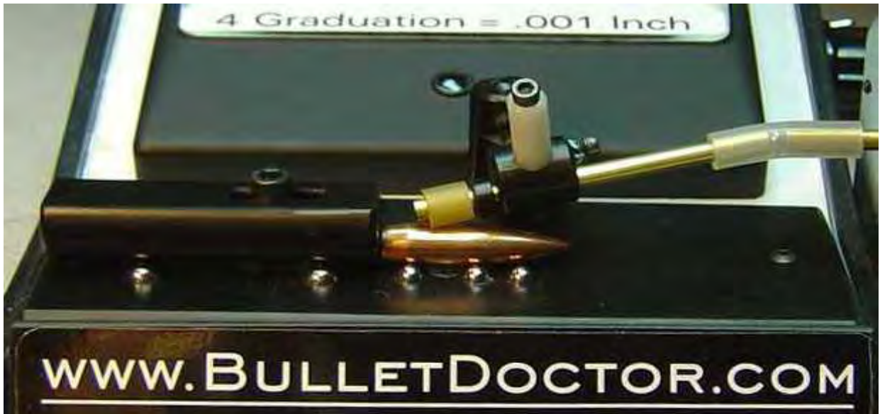
Above: Drive arm is in the down position.
